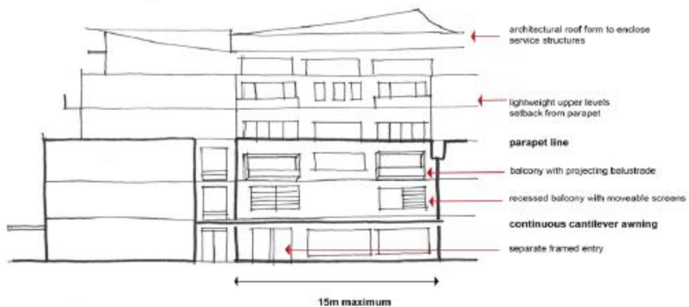
Figure 17 – Building Type C Street Elevation
