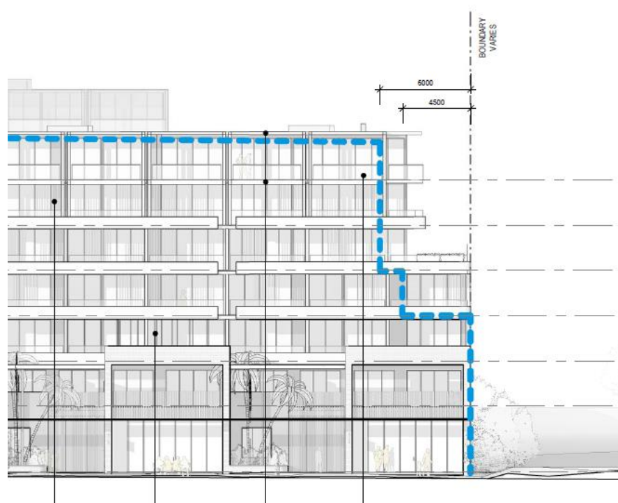
Figure 8: Setbacks under the ADG (blue line)
